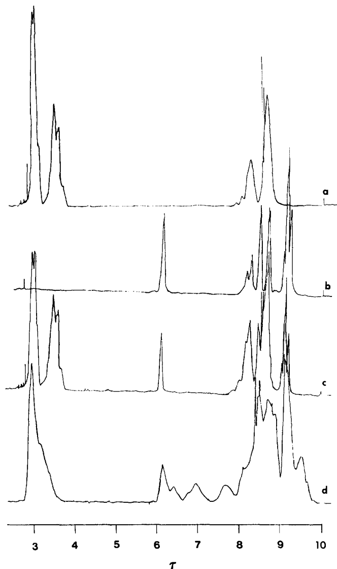
Figure 2 Proton n.m.r. spectra of curve a, polystyrene; curve b, poly(buthyl methacrylate), curve c, polymer blend of equal weight of polystyrene and poly(buthyl methacrylate) prepared by solution blending, and curve d, copolymer of equal weights of styrene and buthyl methacrylate
